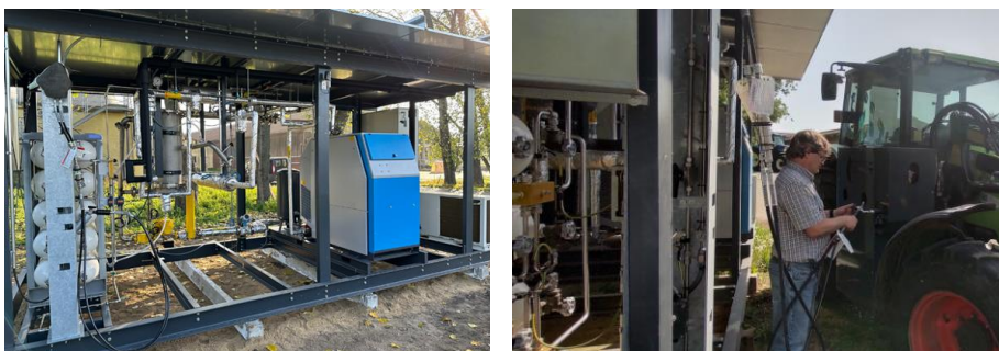
BioCNG upgrade plant and fillig station (left), filling up a CNG tractor (right)
