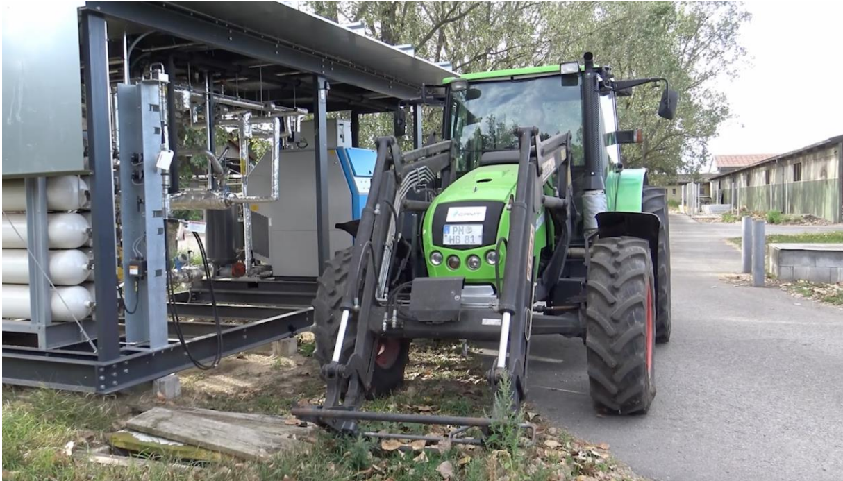
Figure 4. Snapshot from the RES4LIVE final video showing the retrofitted tractor and the BioCNG station at LVAT dairy farm, Germany.
