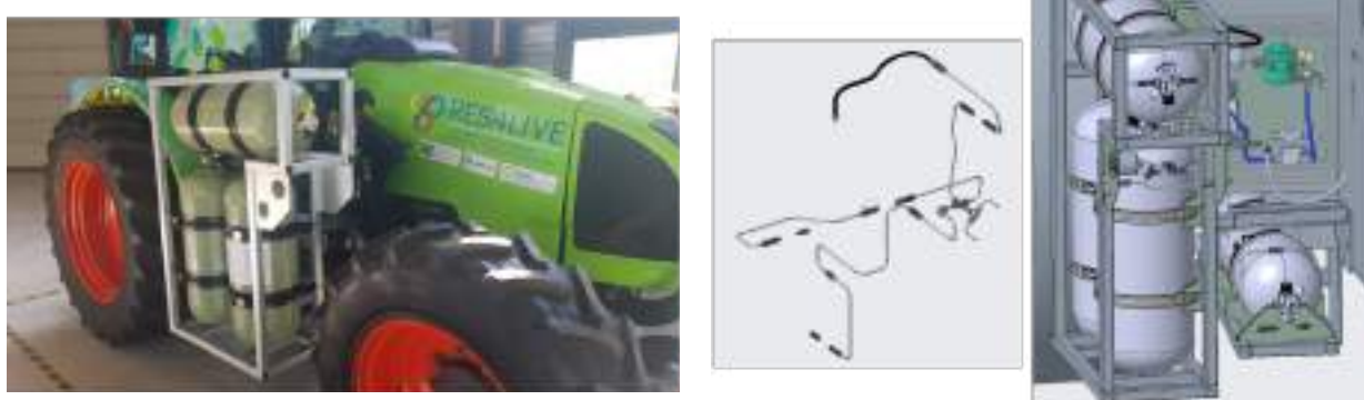
Gas tanks on the tractor and gas pressure regulation system
