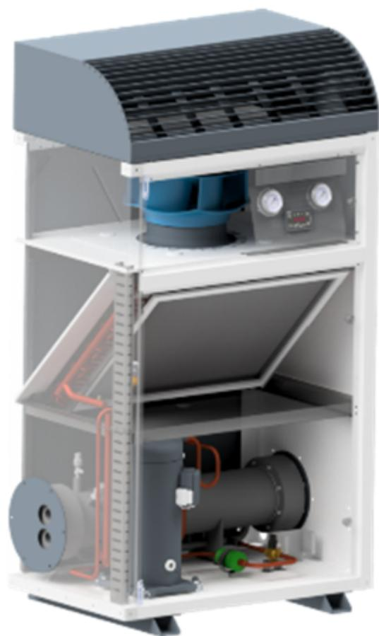
They can draw energy from ambient air or water (coming from ground or solar collectors) to heat internal air (typical A/C heating mode) or provide hot water (35-50 °C). In cooling mode energy is extracted from hot spaces by circulating cold water or air with a piping system, in order to lower the comfort temperature of the animals (15-25 °C).
