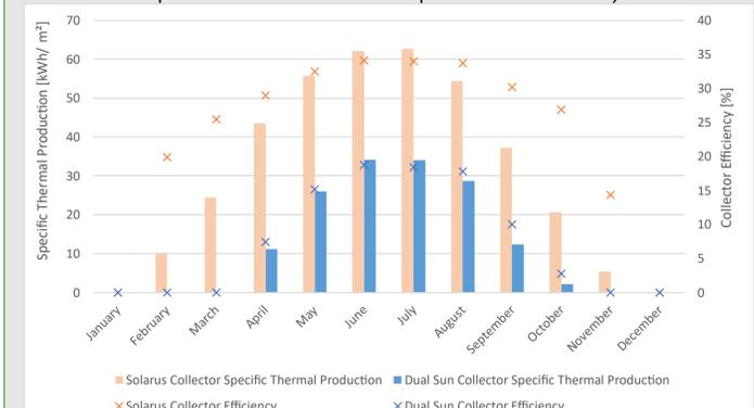
Figure 4. Specific thermal production and collector efficiency at collector mean temperature of 45°C (Inlet=40 °C and outlet=50°C) for total aperture area of 40 m<sup>2</sup>
