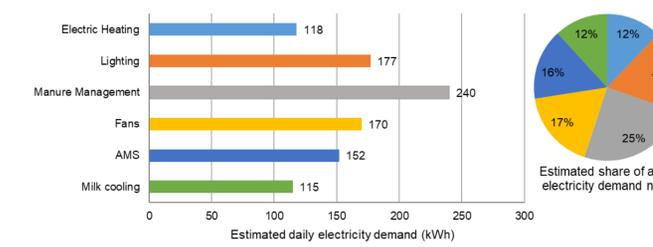
Figure 3. Estimated daily electricity demand breakdown and percentage of annual electricity demand for each application at LVAT-ATB in Germany.
